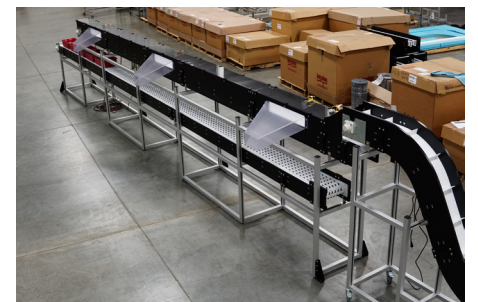
Multi-stack conveyor solution with three sort/divert stations.
