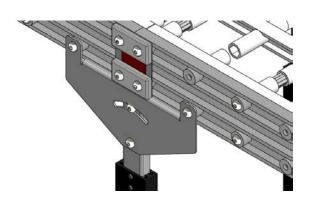
Adjust the height by removing the screws in the upright bracket and sliding the conveyor up or down to the desired height
