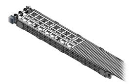
When the belt reaches the drive module make sure that the sprockets engage the belt correctly and wrap the belt around to the underside of the conveyor going over all the return rollers
