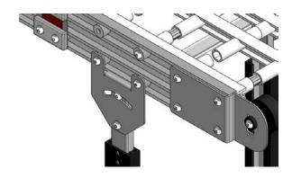
The leg sets that are connected to the mid module will be larger and will connect between 2 mid modules.
